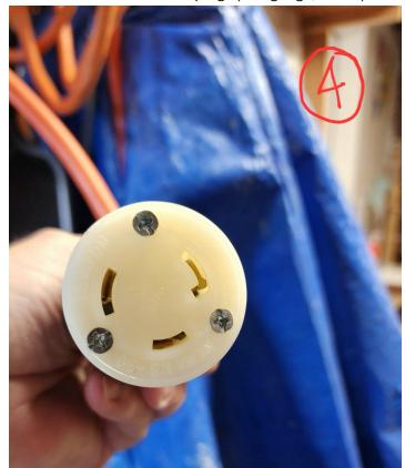
ii. Power cord with twist-lock plugs (#10 gauge, 3 wire)
