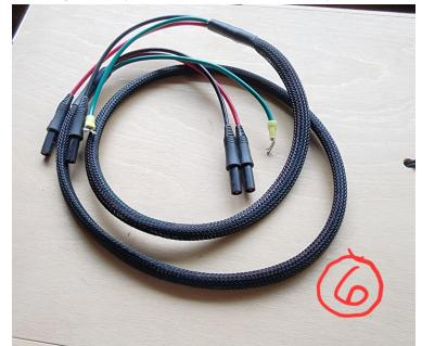
iv. Patching cables (comes with Companion Gen.) to connect the 2 generators
