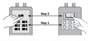
Circuit Box with Shut-Off Step 1: Shut off individual breaker.
