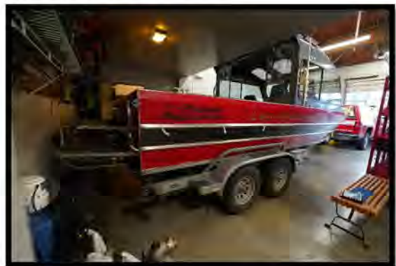
Figure 6. The rescue boat fits in the apparatus bay with less than three inches of clearance.
